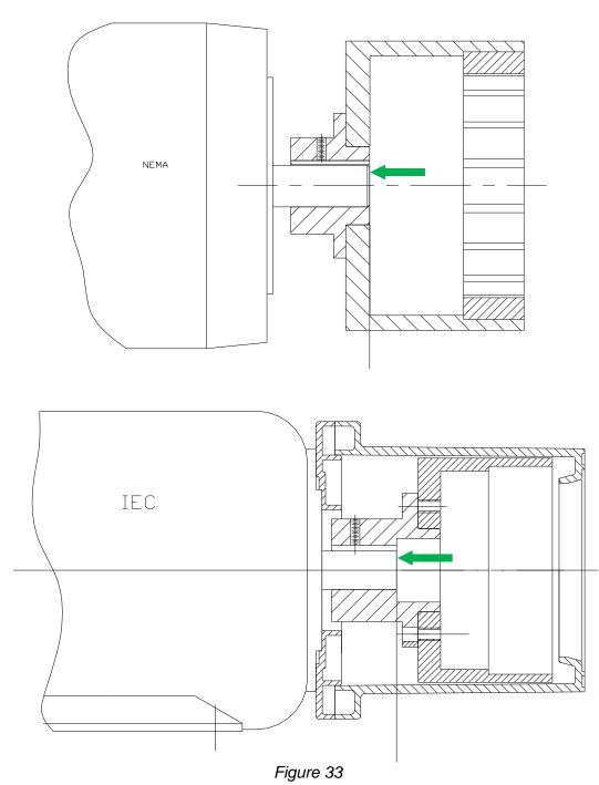
(item 26). Application of a no-seize compound on the shaft and key will make future maintenance easier.
