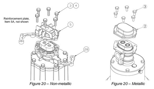
4. Remove bearings, gear/shaft assemblies, and housing liner as shown. These parts, along with the four o-rings make up a standard Eclipse Series KOPkit. Check parts for wear and replace with a KOPkit as required.
