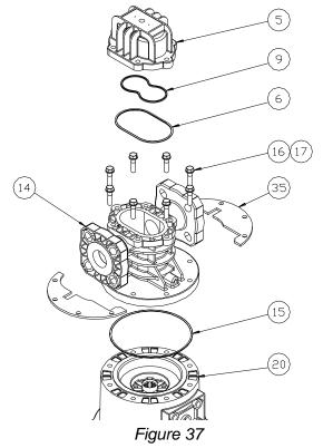
8. Remove driven magnet assembly (item 21) and containment can (item 19) from the motor spool (item 20) as shown.
