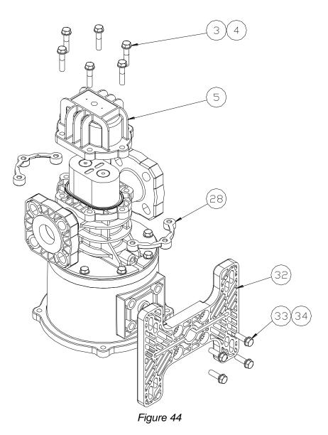
11. Secure the mounting base (item 32) to the motor spool (item 20) using the four bolts and washers (items 33, 34) as shown. Always tighten fasteners in a progressive "crisscross" pattern.
