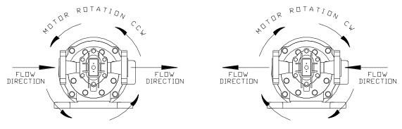
Figure 2b – Flow vs. Motor Rotation
