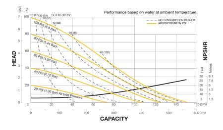
MAX CAPACITY 150 GPM (568 LPM)
