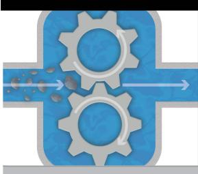
While **gear pumps** can move clean, clear fluids effectively, they lack the ability to handle solids and fluids without lubricity. Historically, gear pumps have been used to pull tank bottoms which commonly see the presence of water and sand; greatly shortening the life of the pump.
