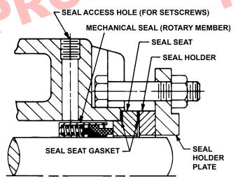
FIGURE 5 - PTFE FITTED MECHANICAL SEAL
