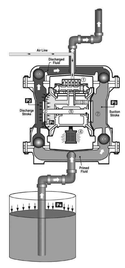
VERSAMATIC e1nmdlCsmPM-rev1219 The main directional (air) control valve ① distributes compressed air to an air chamber, exerting uniform pressure over the inner surface of the diaphragm ②. At the same time, the exhausting air ③ from behind the opposite diaphragm is directed through the air valve assembly(s) to an exhaust port ④.
