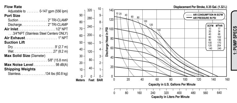
NOTE: Performance based on the following: flooded suction, water at ambient conditions. The use of other materials and varying hydraulic conditions may result in deviations in excess of 5%.
