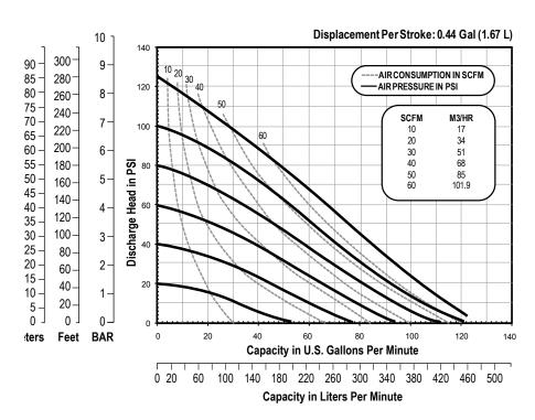
NOTE: Performance based on the following: elastomeric fitted pump, flooded suction, water at ambient conditions. The use of other materials and varying hydraulic conditions may result in deviations in excess of 5%.
