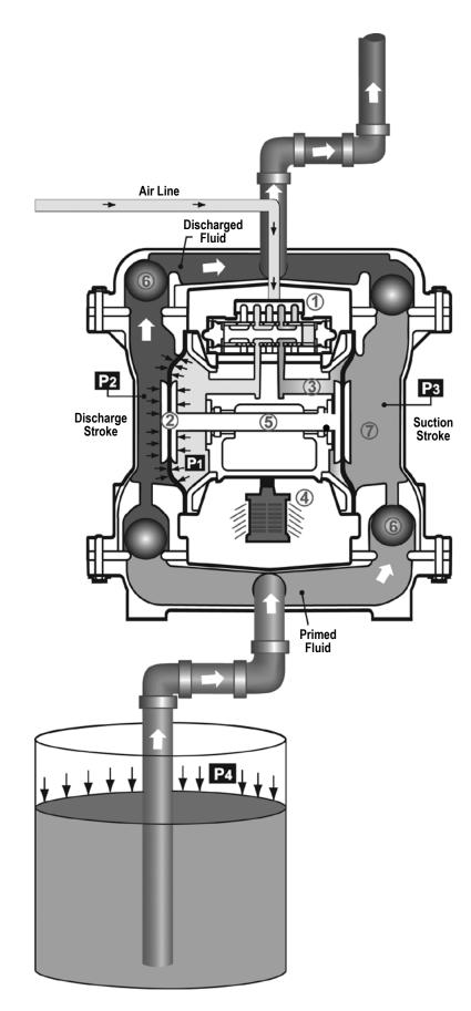
versamatic – e6nmdlCsmATEX-rev0420 Air-Operated Double Diaphragm (AODD) pumps are powered by compressed air or nitrogen.
