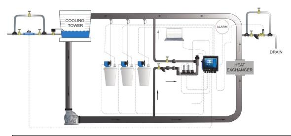
Over pressurization of the plumbing can occur when cooling tower is higher than the piping and controller system. Ensure all pressures have been accounted for. Verify piping and sensor allowable temperatures are above maximum temperatures of the system.
