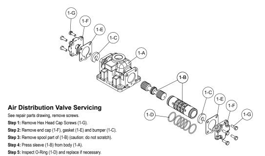
Step 6: Lightly lubricate O-Rings (1-D) on sleeve (1-B).
