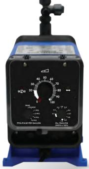
Built on the proven PULSAtron Series pump platform, E+ Ratio Control (RC) offers manual control over stroke length, automatic speed control based on a water meter input signal and a selectable ratio control from 0.1 Oz/ Gallon to 1.0 Oz/ Gallon.
